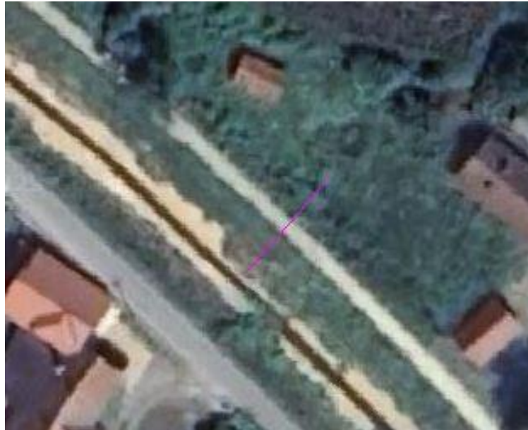
Figure 2.43: Tentative estimate of dike rate width using Google Satellite in RAS Mapper
