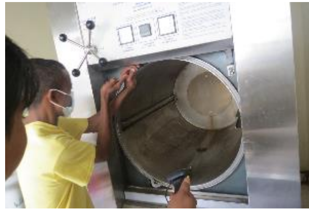
Replacing the door gasket of JSD 260
